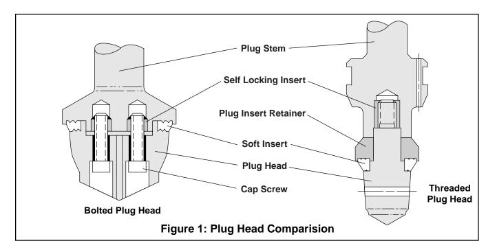
of the plug stem. A rod may be inserted into the hole drilled through the plug head to facilitate removal. Plugs above 2 inch use a bolted design that clamps the soft insert between the plug head and plug stem. Disassemble the plug by removing the cap screws.
